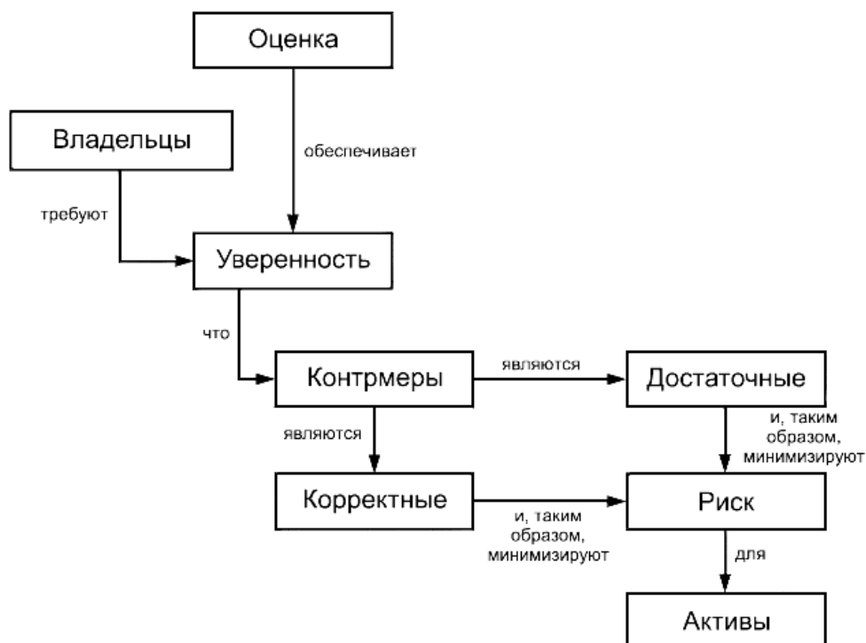
Fig.2. The concept of cybersecurity in the context of risk-based approach to protect assets of business owners Source: ISO/IEC 15408-1-2012 [5]
